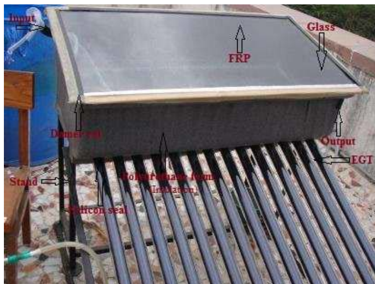
Fig. 8 Solar still coupled with Evacuated glass Tubes [2].
